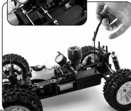
Do not extend fully the pull start beyond. Keep the extension to around 20cm with short sharp pulls.
