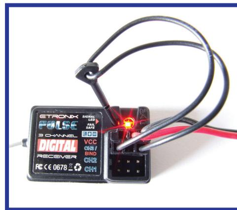
**Once the 'Bind' process is complete, the throttle failsafe position can be set by pressing the button using the pointer provided.**
