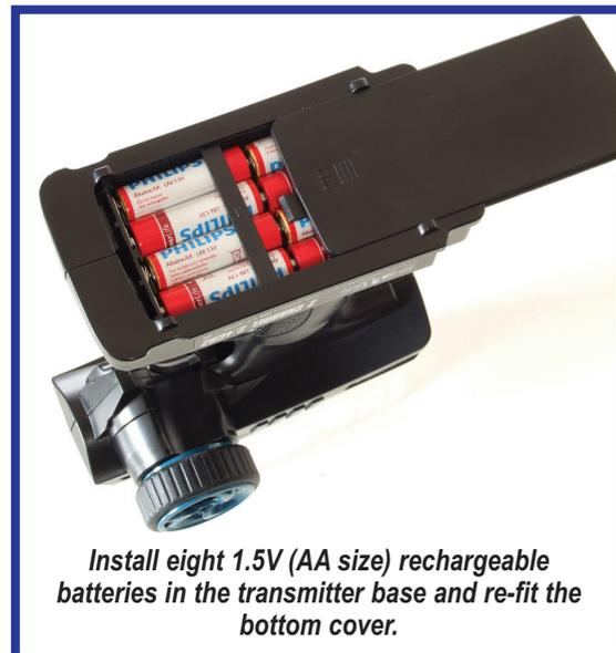
Install eight 1.5V (AA size) rechargeable batteries in the transmitter base and re-fit the bottom cover.
