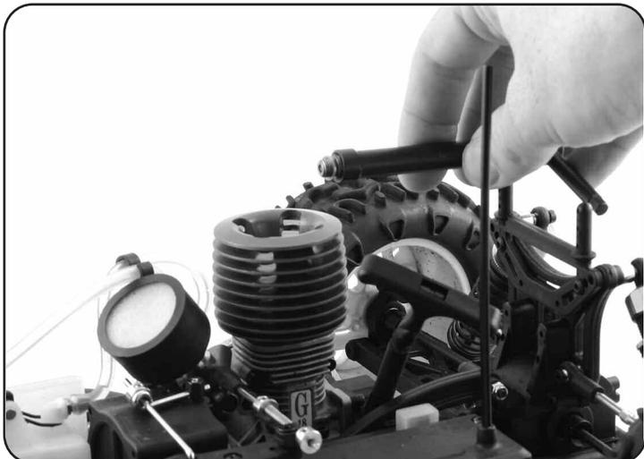
3. Start engine. Add fuel to the fuel tank using a suitable fuel bottle. Use a glow plug heater to ignite the engine plug as illustrated and start to pull the the pull starter (be careful not to extend too far as mentioned previously). Ensure you have a small amount of carburetor open (around 2mm) to allow for air intake to help starting.
