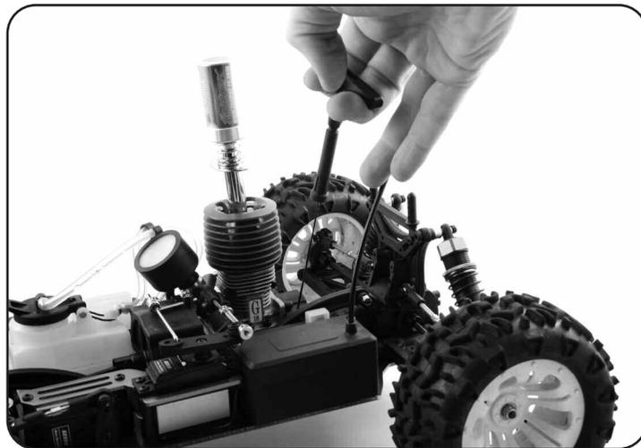
The engine will run “lumpily” or stop after a few seconds so try and keep it running by blipping the throttle. Tighten the glowplug while the engine is running if possible. If the engine has stalled restart with the plug tightened. The above procedure should always be followed from cold or if difficulty with starting is being experienced.
