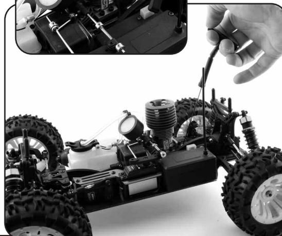
Do not extend fully the pull start beyond. Keep the extension to around 20cm with short sharp pulls.
