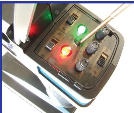
**With the power on you can release the bind button once the green LED begins to flash to indicate the "Bind" process has initiated.**
