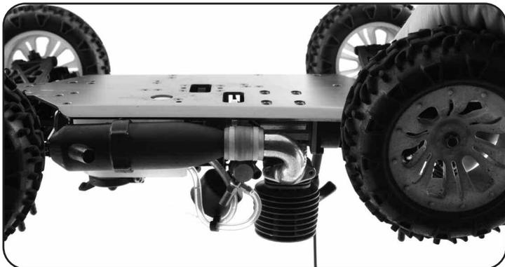
2. Then turn the car upside down and pull the pullstarter rapidly until all the excess fuel has emptied onto the floor through the glowplug hole. Make sure you do this outside safely. This process is really only necessary when the engine is cold or brand new and tight.
